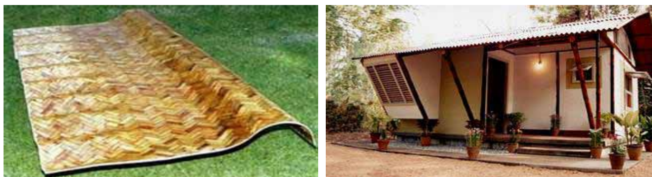
Figure 10: Bamboo Mat corrugated sheet and bamboo house (Source: BMTPC, IPIRTI)
